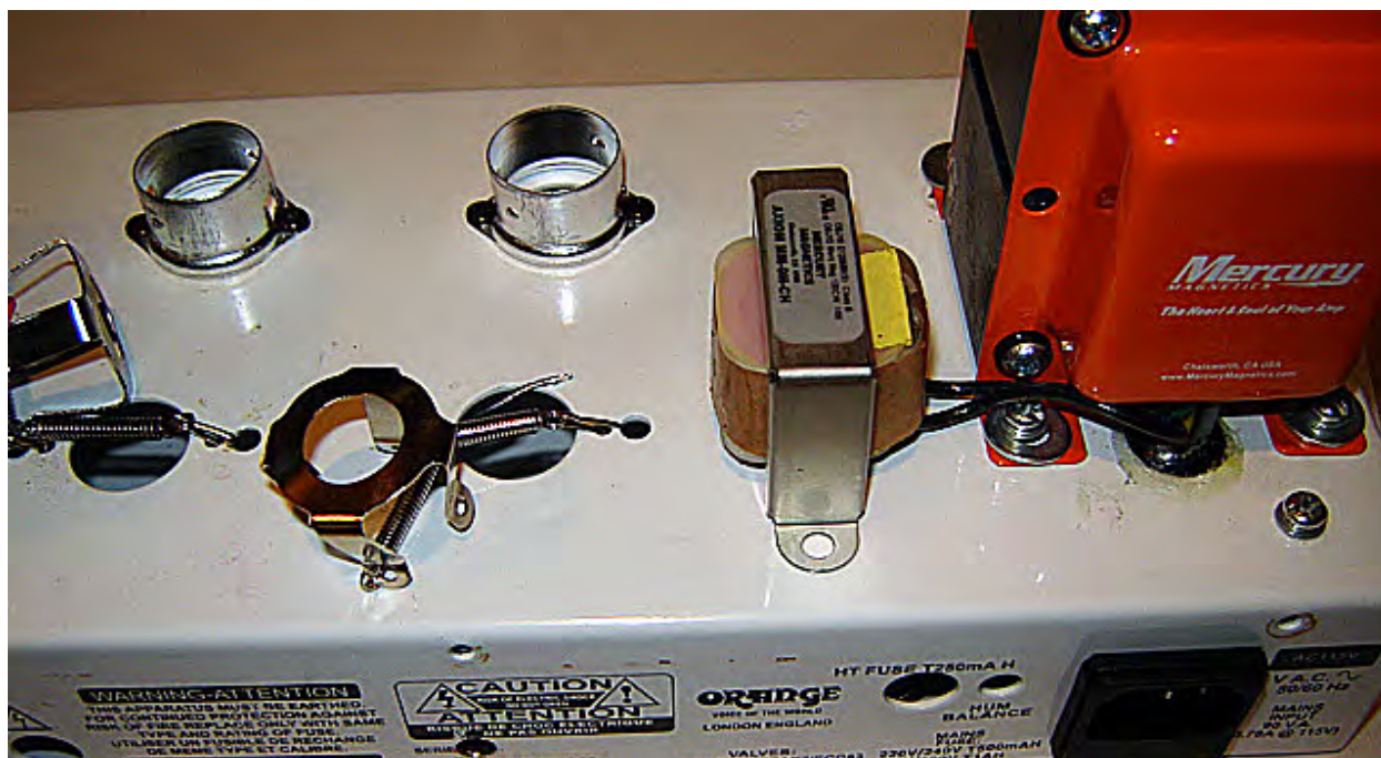
Picture 5: The Mini-Choke leads will fit through the existing hole used for the Power Transformer's leads. Mount your Mini-Choke and carefully pull the leads through that hole.
