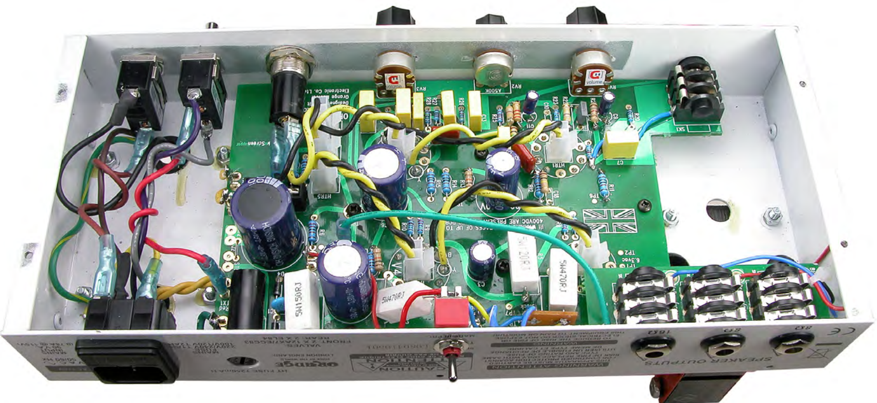
Chassis reference photo: A fully reassembled chassis (version 1, 2 & 3). Note that lead colors and standoff to PTS are different than description in manual.
