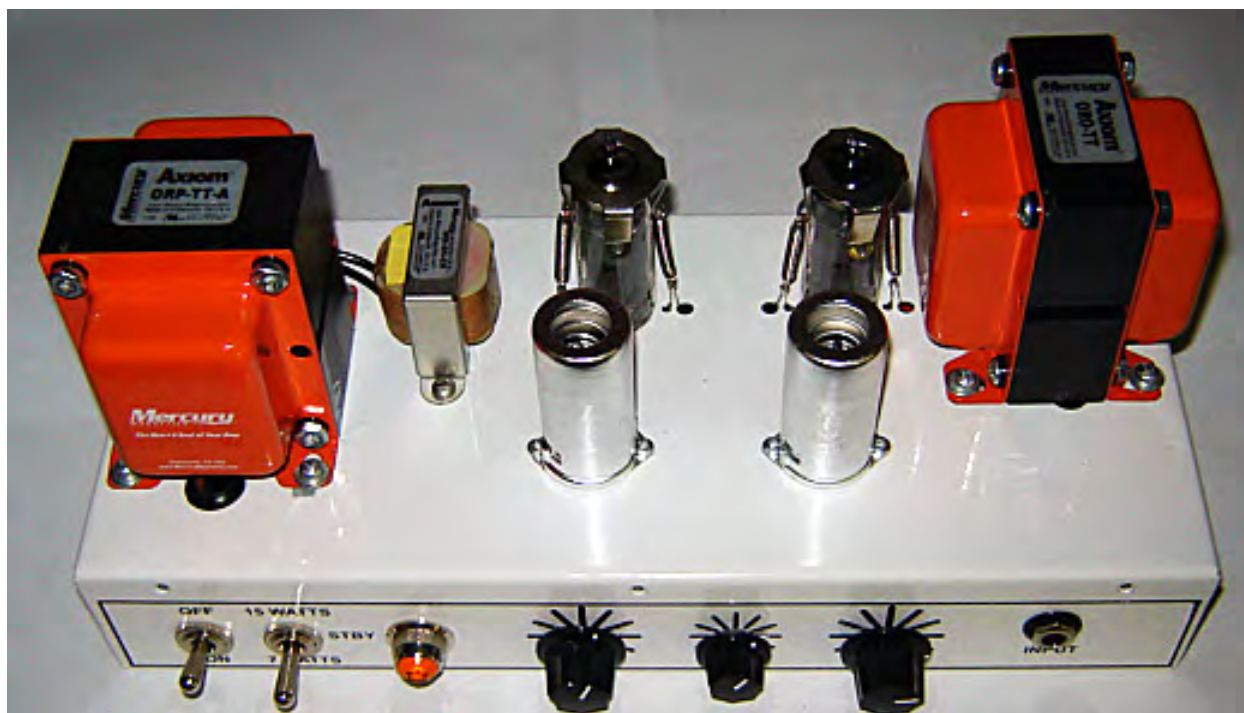
Picture 6: The chassis with the new Transformers and the Mini-Choke in place looks great!
