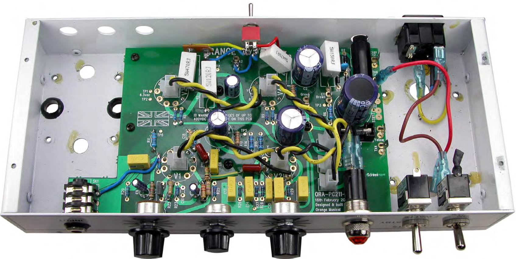
Chassis reference photo: A fully modified main PCB (version 1, 2 & 3). Note that lead colors and standoff to PTS are different than description in manual.
