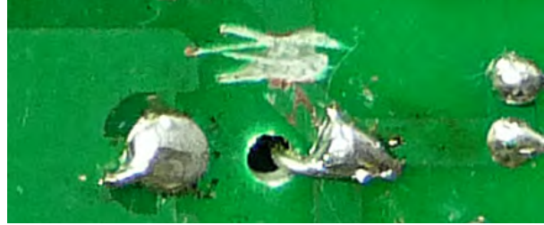
Various examples: This photo shows a cut trace, and a component lead jumpered and soldered to a revealed trace. It's best to not drill a hole directly into a trace. Instead make the hole off to the side of the trace and then, as in this example, solder the component's leg to the trace.
