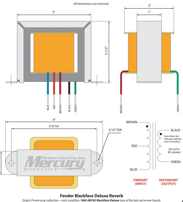
CLASS: ToneClone® TYPE: Output Transformer PART NO.: FBFDR-O ORIGINAL FENDER PART NO: 125A1A MOUNTING: A-Frame / Horizontal Mount **RECOMMENDED TUBE TYPES**: two 6V6 or EL84/6BQ5 **POWER RANGE**: Our OTs are rated to handle up to 50% more power than the original manufacturuer spec. **DATE**: 01-27-06/10-13-06
