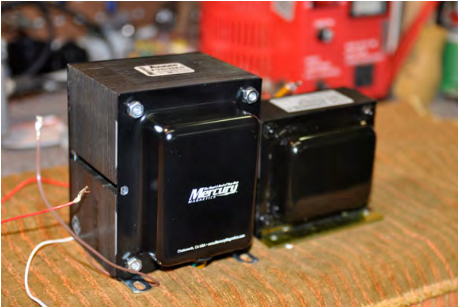
Mercury's replacement compared to the stock output transformer!
