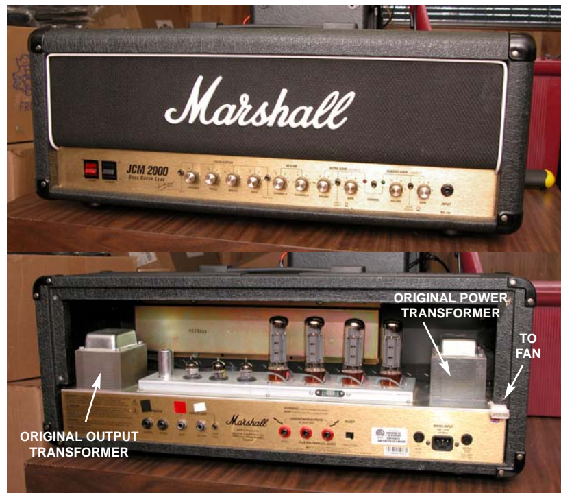
BEFORE: Front and back views of JP's unmodified Marshall JCM 2000 Dual Super Lead . Note the fan connector next to the power transformer . JP was experiencing overheating issues due to the undersized original transformer .
