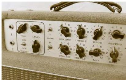
The *Lead* channel controls function much like an overdrive pedal, with *Drive*, *Level* and *Tone* controls and a toggled *Boost* switch. A *Midrange* control is also included. You couldn’t ask for a clearer, more intelligently designed control panel, and the controls themselves are simple and intuitive. As with many overdrive or boost pedals, mixing variable settings for *Drive* and *Level* pro-
