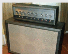
Back in the day, if the Silvertone 1484 wasn't enough, you could crank up its big brother—the mighty 1485. This beast sported six Jensen 10" speakers and pumped out 120 watts of vintage tube tone. Photo courtesy of Fargen Amplification
