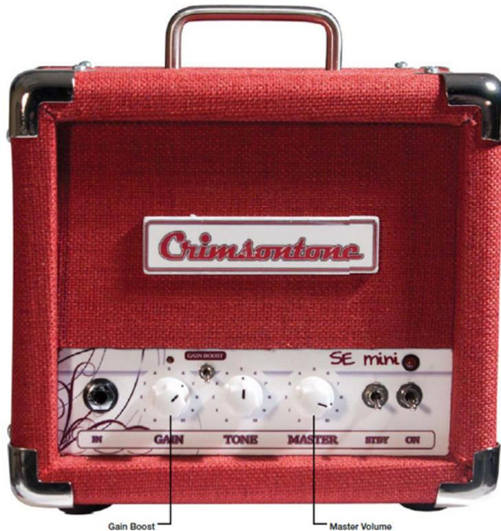
The single-ended all-tube head is powered by a Sovtek EL84 coupled to a JJ ECC803 preamp tube and a **Mercury Magnetics** GA5-P power transformer for a maximum of four watts.
